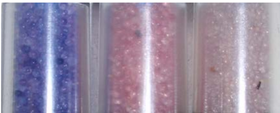
Desiccant stages (from left) New, nearly expired (replace now), expired
