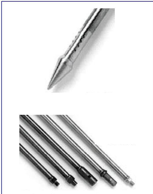
Supplied as a set of parts for sampling to depths of about 4' (1.2m) by hand using the supplied cross handle. This gas vapor probe may be used to probe to greater depths using additional extensions and the Slide Hammer available separately.
