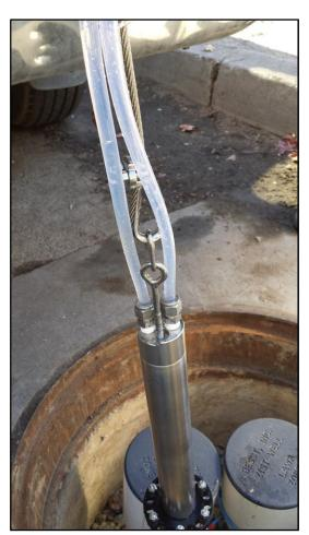
Figure 2- Stainless Steel Panacea P200 being deployed into a nested monitoring well in North Hollywood, CA. Tubing is 3/8" OD FEP bundled with 3/16" stainless steel support cable. The docking cage is located at the bottom of the photo.
