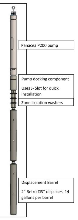
Figure 1 - Model of the Retro ZIST system for a 2" well using two displacement barrels stacked to fit length of well screen.
