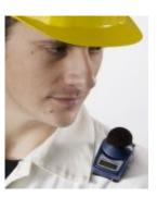
all standard dBadge kits are provided with a charger and slave charger(s) to suit the number of dBadges selected plus; infra red interface, dB35 database software, USB to RS232 adaptor, 110/240Vac to 12Vdc universal power supply, acoustic calibrator, pin and alligator clips and a carrying case to fit up to 12 dbadges and accessories
