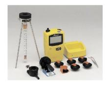
The Pump Manager software is available for use with the logging functions of the Apex Pro model and handles all the setup and downloading of relevant pump data for comprehensive archiving. A drop in fast charger intelligently charges the Apex pumps and maintains them at peak readiness for a new measurement. An optional dry cell battery pack is also available for those really urgent jobs when there is no time to recharge a unit prior to use.
