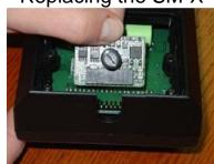
When the sensor needs to be replaced it is a very simple process. This image shows the SM-X being installed into the A-22 Ozone Sensor.
