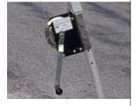
The EZE-MAN Winch is a Suspension (SU) and Retrieval (RT) unit designed to be used in conjunction with the EZE-MAN Tripod. It functions by lowering and raising a worker into and out of confined spaces with ease. The EZE-MAN Winch does not provide Fall Arrest (FA) protection. A personal fall arrest system is required whenever a worker is being raised or lowered more than six feet.
