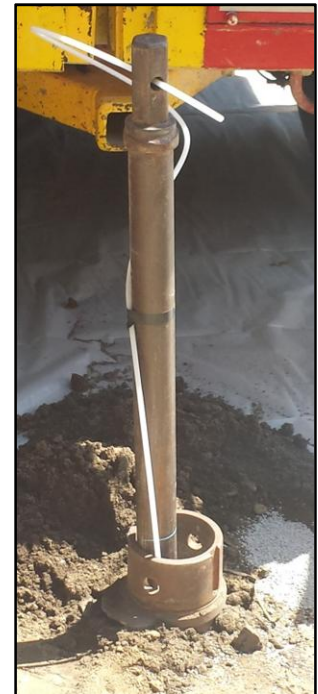
Figure 1 - Mini Probe deployed in hollow stem augur.
