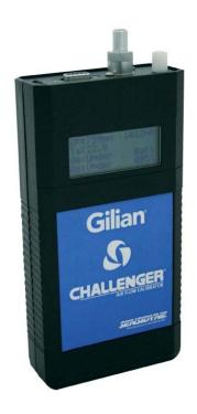
Introducing the Challenger air flow calibrator for verifying and calibrating Industrial Hygiene Air Sampling Instruments and other air sampling devices. The Challenger is accurate within 0.75% of reading and provides a LCD indication of Volumetric and Standard flow rate, barometric pressure and ambient temperature.
