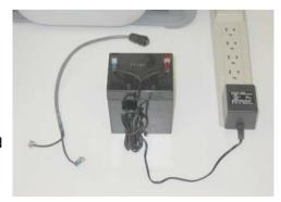
NOTE: The battery life will last longer if recharged before it drains below 10.5 volts.
