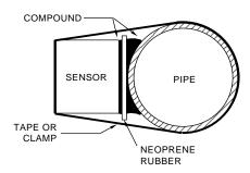
SENSOR POSITIONING - The sensor must be mounted away from velocity increasing devices such as pumps, controlling valves, orifice plates, venturis, or pipe inlets and discharges. These devices cause release of gas bubbles in the fluid and readings nearby will indicate higher velocity. Normally flow will be evenly distributed 30 to 40 pipe diameters away from the velocity increasing device. Determine an appropriate up or downstream sensor mounting location by onsite experimentation.
