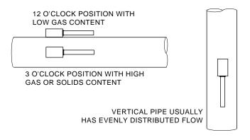
*FLOW VELOCITY* - Doppler accuracy and signal strength is reduced at very slow velocities (1.0 ft/sec, 0.3 m/sec or less). Engineers usually design piping systems for velocity in the 2-10 ft/sec (0.6 -3 m/sec) range which is ideal for Doppler instruments.
