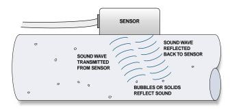
The advanced DFM sensor contains two piezoelectric crystals in a stainless steel housing. One crystal transmits ultrasonic pulses at a precise frequency which are reflected back to the receive crystal from gases or solids in the liquid. Because the fluid is in motion the returned echo arrives back at the sensor at an altered frequency (called the Doppler effect). The instrument's electronics monitor and convert this frequency change into velocity flow readings.
