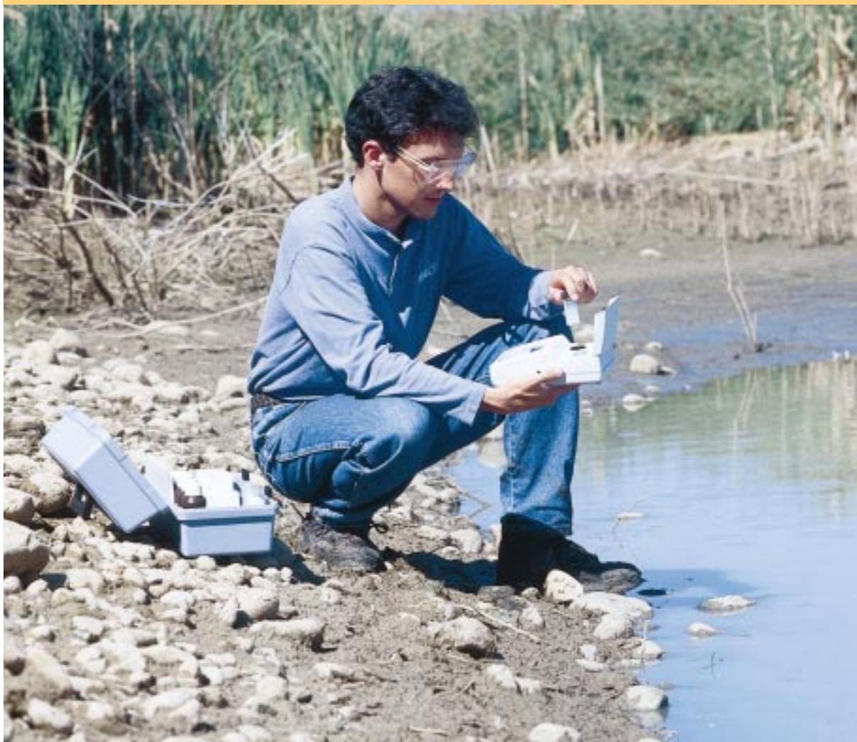
The 2100P Portable Turbidimeter offers a level of performance previously possible only with laboratory instruments. The 2100P combines microprocessor-controlled operation and Hach's patented Ratio™ optics to bring greater accuracy, sensitivity, and reliability to field testing.
