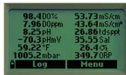
**Fully Configurable Measurement Screen**
