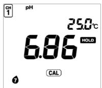
The measured value will be displayed, and "HOLD "will blink until the reading stabilizes.
