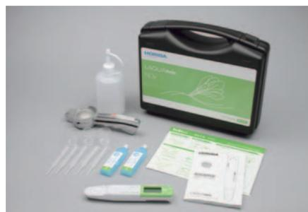
■ Measurement range: 100 to 9,900 ppm (NO<sub>3</sub><sup>-</sup>)
