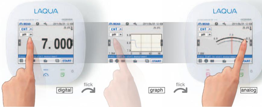
Two channels can be displayed simultaneously
