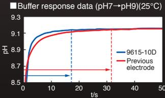
Our proprietary glass purification technology ensures high speed and stable measurements with low-conductivity samples
