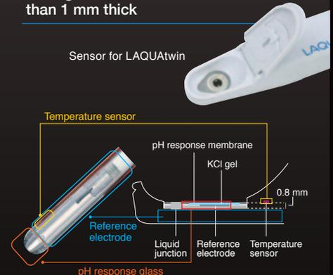
Glass electrode components contained in a flat body of less than 1 mm thickness allows measurement by directly applying a drop of the sample onto the flat electrode instead of dipping the electrode into a beaker. Thus, the LAQUAtwin can measure minute volumes down to just 0.1 mL, and various sample types including solid materials containing moisture, powders, and sheet materials.
