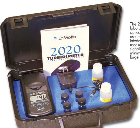
The 2020 sets the new standard for laboratory accuracy. With a multi-detector optical configuration, long term stability is assured and stray light and color interferences are minimized. Rapid, reliable measurements are obtained by averaging signals over a 5 second period, which minimizes fluctuating readings attributed to large particles.
