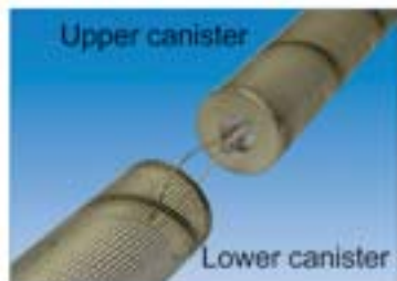
Detail showing how two canisters are linked. Up to three canisters may be suspended in line to lengthen the active zone.
