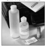
Easy-to-use replacement membrane assembly—simply fill with electrolyte solution and screw onto probe.
