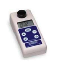
The OAKTON T-100 turbidity meter is easy to calibrate-meter automatically prompts you to the next calibration standard. The large custom LCD displays reading and units of measure. Other features include auto-off, diagnostic error messages, and auto-ranging function. Power saving function lets you take over 1000 readings on a single set of AAA batteries. Sealed optical system with infrared light source delivers high accuracy across entire range.
