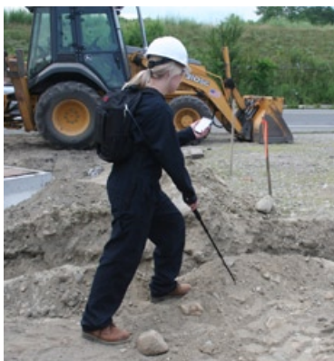
MicroFID II with telescoping probe, backpack and handheld computer.
