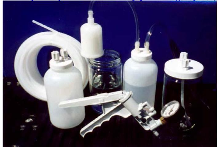
All transfer vessels are pre-cleaned to EPA protocol "B", and individually packaged in a poly bag.
