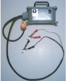
guidelines. Simply hook the controller to a car battery and connect the pump to the Contoller, turn on device with the on/off switch on the side and sample with total control over the pumping volume.
