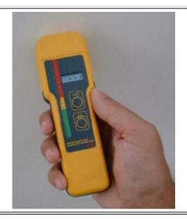
**Measure Mode** gives a precise moisture level value in wood and other building materials from pin electrodes or deep wall probes.
