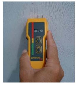
**Heavy Duty Moisture Probe** -supplied standard with the Surveymaster SM.
