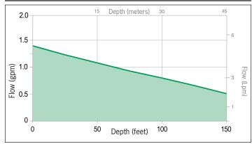
Curve generated using supplied voltage booster and 150 ft. (45.7 m) of power cable and tubing. Results may vary depending on actual field conditions, frictional line loses, battery capacity, and amperage draw.
