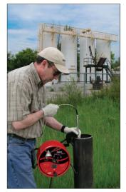
If the liquid is a non-conductive oil/product the signals are steady. If the liquid is water (conductive liquid greater than 20  $\mu$ S/cm), the conductivity of the water completes a conductivity circuit. This overrides the infra-red circuit, and the tone and light are intermittent.
