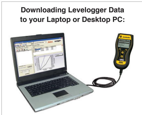
You can download Levelogger readings from your Leveloader to your desktop or laptop PC, using a USB or RS232 Communication Cable and Levelogger Software. You can also create and save up to 10 customized Levelogger settings files for transfer to Leveloggers in the field.
