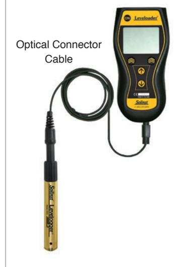
If you have deployed your Levelogger using wireline/cord deployment, remove your Levelogger from the well, and program, view or download data in the field using an Optical Connector Cable.
