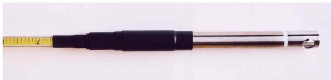
small diameter wells. This provides unparalleled accuracy when compared to the flat white tapes, where kinks in the tape introduce slight errors, in addition to the displacement of water changing the static level.
