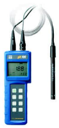
The new YSI pH100 depicting one of the possible configurations with a combination 3-in-1 pH sensor and temperature sensor. Another option allows for a mV or pH sensor with a separate temperature sensor.
