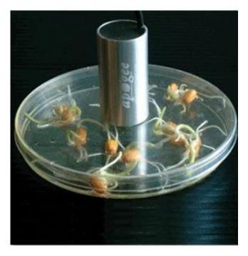
Apogee oxygen sensors are resistant to 2.7 G of shock, but vibration may influence sensor sensitivity and should be minimized.
