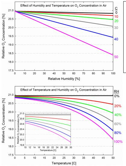
A) Relative humidity effects on relative oxygen concentration shown as a function of relative humidity at temperatures increments of 10 C and B) as a function of temperature at relative humidity increments of 20 %. The air in soil is typically always saturated with water vapor (100 % relative humidity) unless the soil is very dry.
