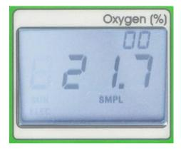
The LCD display consists of the total number of logged measurements in the upper right hand corner, the real-time percent oxygen concentration in the center, and the selected menu options along the bottom.
