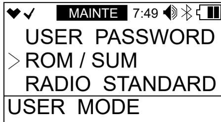
2. Press and release **POWER MODE**. The screen will cycle through the ROM/SUM of the main board, the ROM/SUM of the sensor board, the ROM/SUM of the IR sensor (if an IR sensor is installed), and the Bluetooth version. The ROM is the top value and the SUM is the bottom value.
