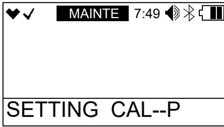
6. Press and release POWER MODE. The combustible gas channel will display.
