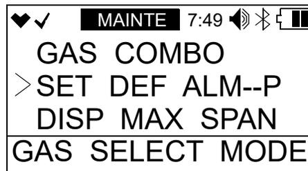
2. Press and release POWER MODE. The display alternate between the following screens.
