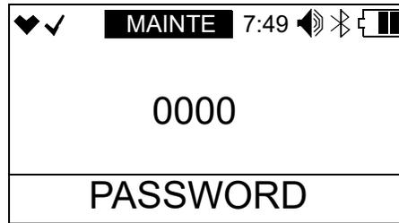
6. Use AIR to select each password number then press POWER MODE to save it and move on to the next number. To go back a number, press and hold AIR and POWER MODE for a few seconds. To reverse the direction of change (ie. from increasing to decreasing or vice versa):
