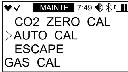
4. Press and release POWER MODE. The Auto Cal screen for gases assigned to Cylinder A will display.
