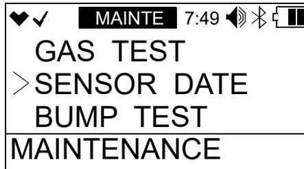
2. Press and release POWER MODE. The combustible gas sensor's replacement date will display.
