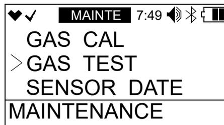
2. Press and release POWER MODE. The current gas readings display. The bottom of the LCD indicates “GAS TEST” and “BUZZER OFF”.
