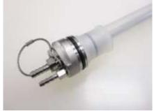
Figure 4-14b: Compression ring secured
