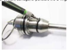
Figure 4-5: Removal of O-rings
