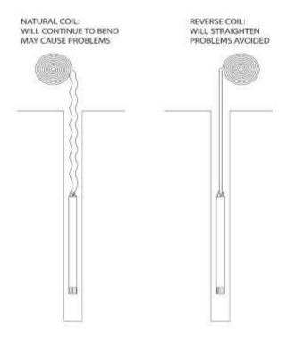
Figure 2-1: Reverse Coil Method
