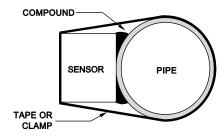
Over time temporary coupling compounds (e.g. Petroleum Gel) may gradually sag away from the sensor resulting in reduced signal strength and finally complete loss of signal. Warm temperatures, moisture and vibration will accelerate this process. Dow Corning Silicone Compound #4 as supplied with the PDFM 5.0 (and available from Greyline Instruments) is recommended for semi-permanent installations.
