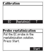
Put the probe into a beaker with replatinization solution and press Start.
