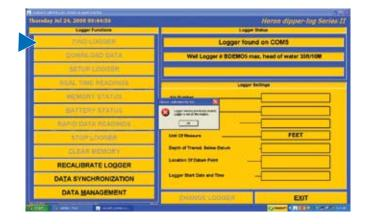
14. Click "SETUP LOGGER" to enter the dipperLog setup screen. Make sure the well Logger is **NOT** in the water at this point.
