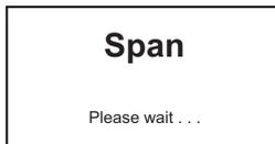
After pressing the **✓** button the instrument will display this message whilst spanning the sensor.
