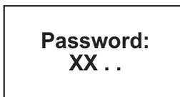
The keys must be pressed in the correct sequence, otherwise the password will be rejected. As each key is entered the '.' will be replaced by 'X'.
