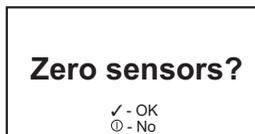
If enabled the instrument will prompt if you wish to zero the sensors in fresh air, to adjust for any natural drift that may have occurred. If the ✓ button is pressed the instrument will then ask the user to ensure that it is being zeroed in fresh, uncontaminated air.
