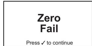
If the zero was unsuccessful repeat the zero ensuring that the instrument is in fresh air. If a second failure occurs the cartridge should be changed. After a successful zero a span should be performed.
