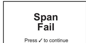
If the span was unsuccessful repeat the span ensuring that the calibration gas used is of the correct concentration, there is sufficient gas in the cylinder and that the flow rate is correct.
