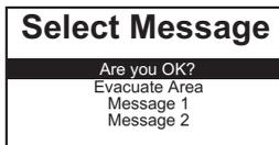
By pressing the ✓ button the Attendant has access to a menu, to select a message to send to the Entrant. These are configurable using the PC software.
