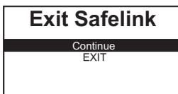
To terminate Safelink mode the cable should be disconnected between the instruments. Both instruments will display a menu enabling Safelink mode to be switched off.
