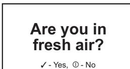
If the ✓ button is pressed the instrument will zero the sensors automatically, and display whether the procedure was successful. The oxygen reading will be adjusted to 20.9%v/v – the other sensor readings will be adjusted to 0 ppm and 0%lel appropriately. If the ⊘ button is pressed instead the instrument will use its current zero values instead and proceed to the monitoring screen.
