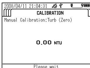
9. When the message "Cal complete. Press ENT to Span cal." appears, press the ENTER key to start the first span calibration procedure.
