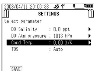
5. If you selected "Input mode", press the right ( ▷ ) key to display the compensation value input screen. Press the up ( △ ) and down ( ▽ ) keys to enter the desired value, then press the ENTER key to set it.
