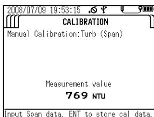
23. Check that "Current measurement value" has stabilized, then press the ENTER key to start calibration.
