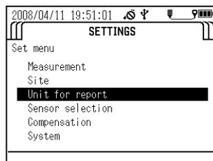
4. Press the up ( ▲ ) and down ( ▾ ) keys to move the cursor to the item to change, then press the ENTER key.
