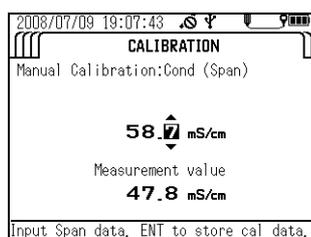
26. Check that "Current measurement value" has stabilized, then press the ENTER key to start calibration.
