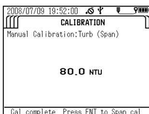
20. Wash the transparent calibration cup 2 or 3 times with deionized water, then fill it to the reference line with 800 NTU standard solution, or a standard solution of known concentration 100 NTU above.
