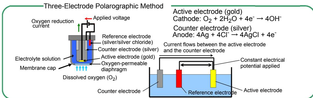
**Fig. 1 Overview of principles behind dissolved oxygen sensor**
