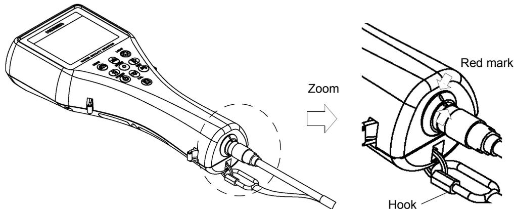
1. Align the red mark on the connector, and press the connector in until you hear it click.
