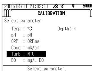
4. Press the up (  $\Delta$  ) and down (  $\nabla$  ) keys to set the number of calibration points, then press the ENTER key.
