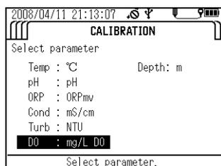
**5. Set the number of calibration procedures, then press the ENTER key.**
