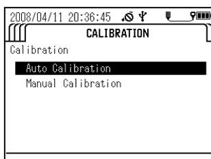
8. Check that the pH sensor, ORP sensor, reference electrode, COND sensor, TURB sensor and temperature sensor are submerged in the pH 4 standard solution, then press the ENTER key.
