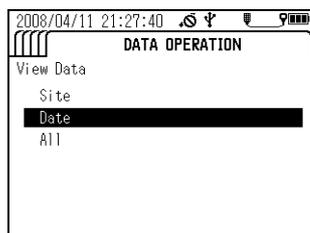
6. Press the up (  $\Delta$  ), down (  $\nabla$  ), left (  $\triangleleft$  ) and right (  $\triangleright$  ) keys to enter the desired date/time, then press the ENTER key to apply the setting.
