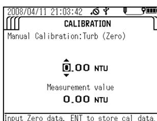
8. Check that "Current measurement value" has stabilized, then press the ENTER key to start calibration.
