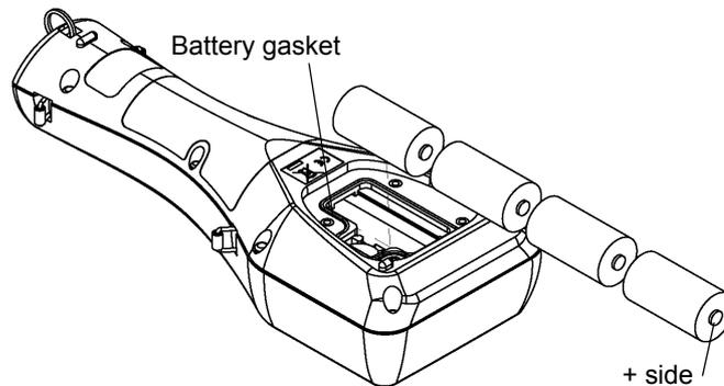
**4. Replace the battery cover and fasten it with the 4 screws.**
