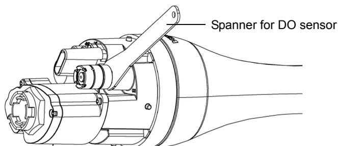
8. Fasten the DO sensor securely using the spanner for DO sensor.
