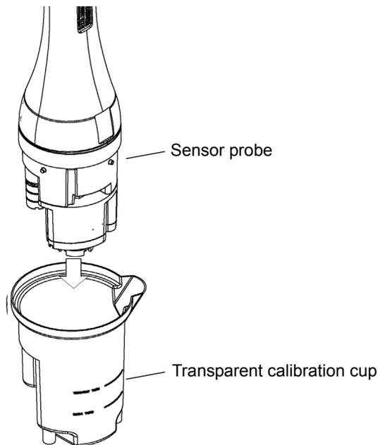
**5. With the sensor probe still in the transparent calibration cup, place the transparent calibration cup into the black calibration cup and start calibration.**
