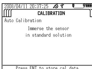
9. When all the sensor values have stabilized, press the ENTER key to start calibration.
