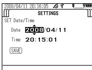
7. When finished entering settings, press the ENTER key to move the cursor to SAVE, then press the ENTER key again to save the settings.
