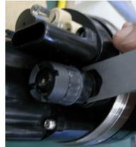
Undo a DO sensor from Sensor Probe
