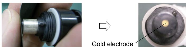
Replace a membrane cap after clean metal electrodes parts.
