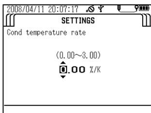
6. To save the change, press the up ( △ ) and down ( ▽ ) keys to move the cursor to SAVE, then press the ENTER key.
