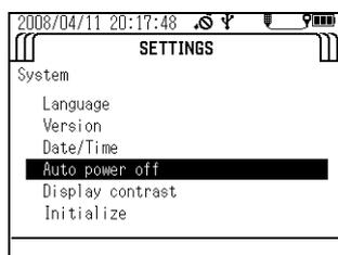
5. Press the up ( ▲ ) and down ( ▾ ) keys to select the desired time setting, then press the ENTER key.
