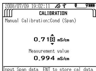
16. Check that "Current measurement value" has stabilized, then press the ENTER key to start calibration.
