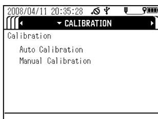
7. Press the down (  $\nabla$  ) key to move the cursor to "Auto calibration", then press the ENTER key.
