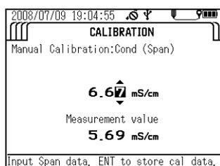
21. Check that "Current measurement value" has stabilized, then press the ENTER key to start calibration.
