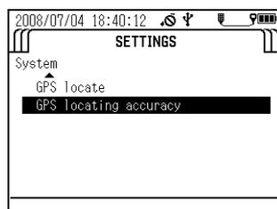
4. The screen below appears. Move the cursor to the locating accuracy, then press the ENTER key. The black circle ( ● ) indicates the currently set precision.
