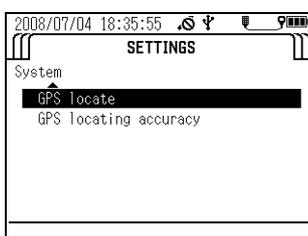
4. The message "Press ENT key to start position measurement." appears. Press the ENTER key.
