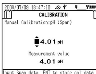
13. Check that "Current measurement value" has stabilized, then press the ENTER key to start calibration.
