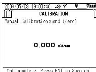
13. Wash the transparent calibration cup 2 or 3 times with deionized water, then fill it to the reference line with 71.8 mS/m (0.718 mS/cm) standard solution.
