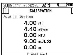
Calibration is finished when the message "Cal complete. MEAS to measure." appears. Press the MEAS key to set the measurement screen, then start measurement.
