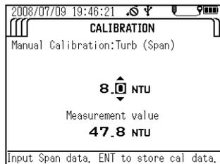
13. Check that "Current measurement value" has stabilized, then press the ENTER key to start calibration.
