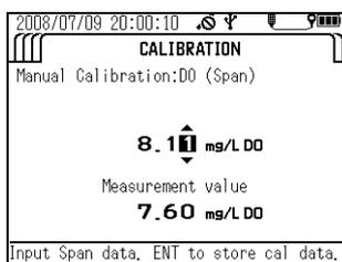
12. Check that "Current measurement value" has stabilized, then press the ENTER key to start calibration.
