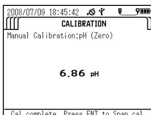
10. Wash the transparent calibration cup 2 or 3 times with deionized water, then fill it to the reference line with pH 4 or pH 9 standard solution.
