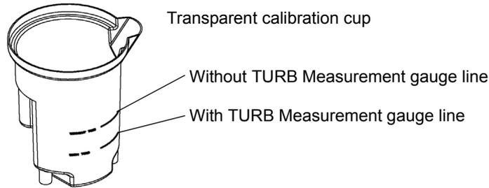
**4. Immerse the sensor probe in the transparent calibration cup, and check that there are no air bubbles on the sensor.**
