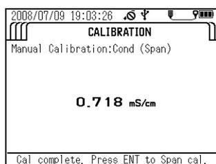
18. Wash the transparent calibration cup 2 or 3 times with deionized water, then fill it to the reference line with 0.667 S/m (6.67 mS/cm) standard solution.
