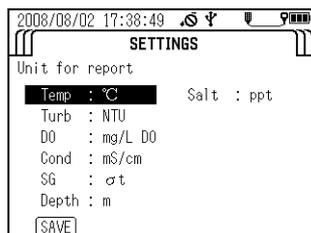
5. A list of the units that can be selected appears. The black circle ( ● ) indicates the currently selected unit. Press the up (  $\Delta$  ) and down (  $\nabla$  ) keys to move the cursor to the desired unit, then press the ENTER key.
