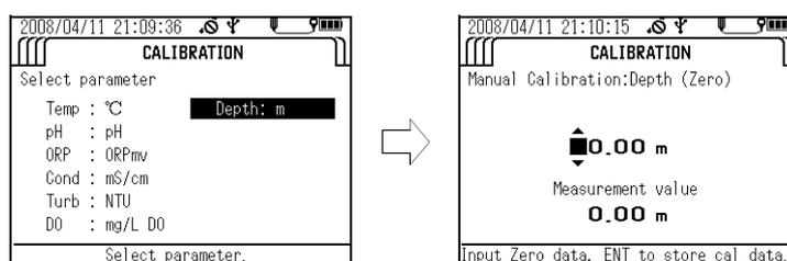
5. Press the up ( ▲ ) and down ( ▾ ) keys to set the "DEPTH" value to 0.00 m.
