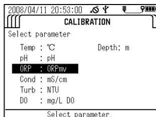
6. Press the up ( ▲ ) and down ( ▾ ) keys to set the mV value of the ORP standard solution containing the submerged sensor probe at the measurement temperature.
