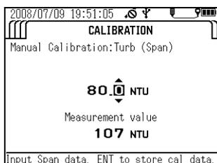
18. Check that "Current measurement value" has stabilized, then press the ENTER key to start calibration.
