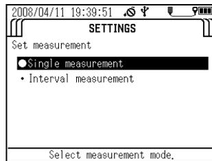
5. If you selected "Interval measurement", the display switches to the screen used to set the measurement interval. Press the up ( ▲ ) and down ( ▾ ) keys to set the measurement interval.
