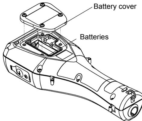
**2. If replacing the batteries, discard the old batteries.**
