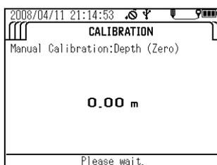
7. Calibration is finished when the message "Cal complete. ENT to manual cal menu." appears. Press the ENTER key to return to the calibration parameter selection screen.
