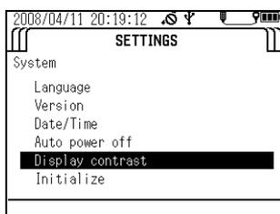
5. Press the left (  $\triangleleft$  ) and right (  $\triangleright$  ) keys to adjust the contrast. Adjustment can be made in 26 steps.
