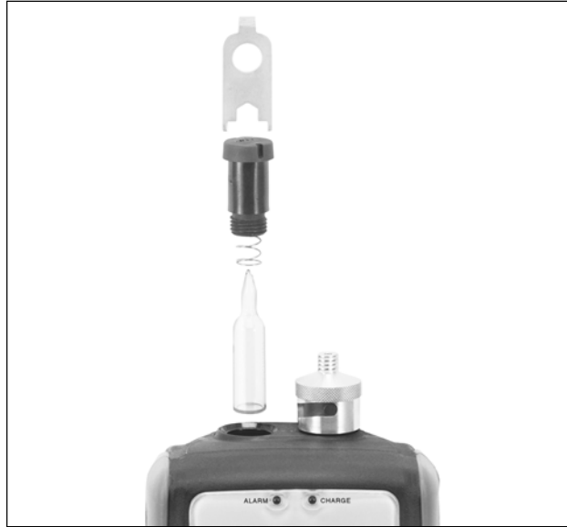
Figure 21. Removing the UV Lamp
