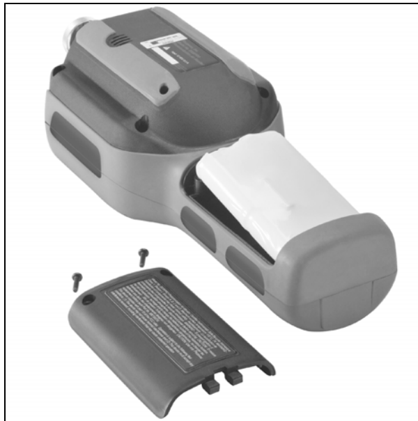
Figure 4. Battery Pack Removal and Replacement
