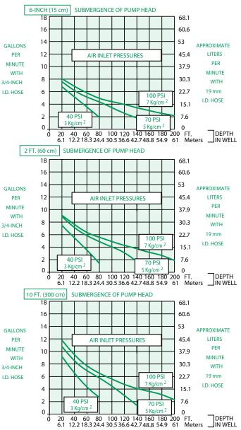
1 inch (25.4 mm) Inside Diameter Discharge Hose (Equivalent to 1.25-Inch O.D. Tubing)
