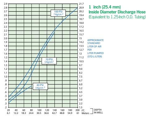
STANDARD CUBIC FEET OF AIR PER GALLON PUMPED (SCF/GAL)
