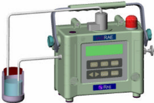
Figure 4-1 Water bubbler connections for span calibration
