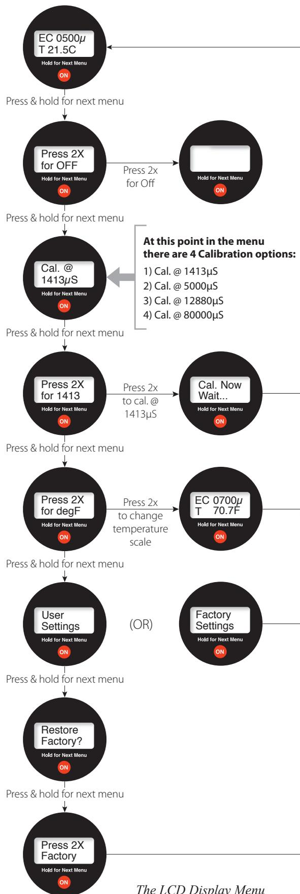
**Note:** To change the temperature scale between  $^{\circ}\text{C}$  and  $^{\circ}\text{F}$ , press and hold the ON button repeatedly until "Press 2X for degF" displays. Press the ON button 2 times quickly to change the scale.
