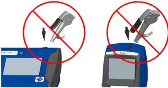
Figure 4-3: Do NOT Blow into Instrument
