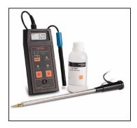
The portable Hanna HI993310 meter measures the soil conductivity in EC (mS/cm) as well as soil activity (g/L). These two measurement modes are made possible using the
