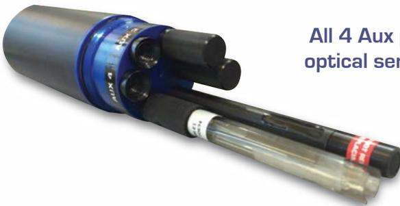
All 4 Aux ports can be fitted with either an optical sensor or an ISE from the list below
