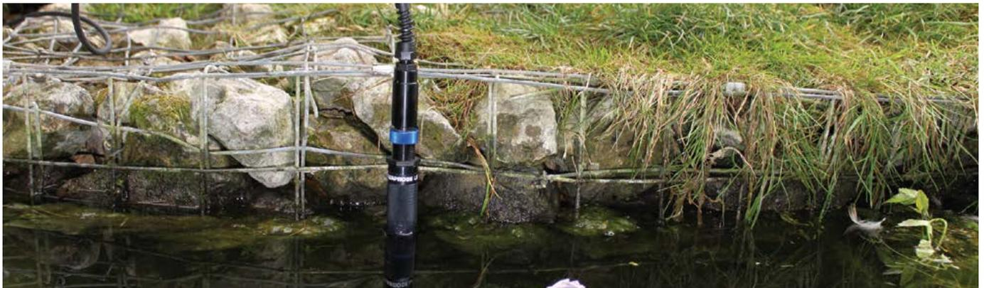
The AP-LITE is commonly used with our sapphire lensed turbidity sensor, chlorophyll sensor or blue-green algae sensors. Whilst the package includes an Aquameter the AP-LITE can also be used with one of our AquaLoggers for unmanned turbidity, chlorophyll or blue-green algae monitoring.
