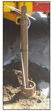
Figure 1 - Mini Probe deployed in hollow stem augur.
