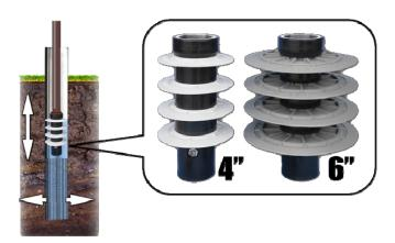
The new Production Series Qwater Well Developer surge block tools fit 4-inch and 6-inch Schedule 40 casing and screens. A check valve in the removable bottom of the tool allows for pumping sediments out of the well while surging. The 4-inch and 6-inch Qwater Well Developers can be used with a wireline (a cable attached to a 10-foot section of iron pipe) or drill rod.
