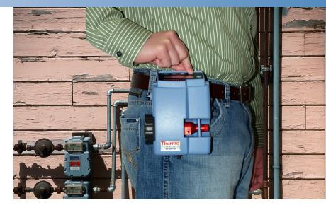
The pDR-1500 personal DataRAM is designed for applications such as site remediation, size discrimination, mass validation, exposure modeling, and protection of asthma patients.
