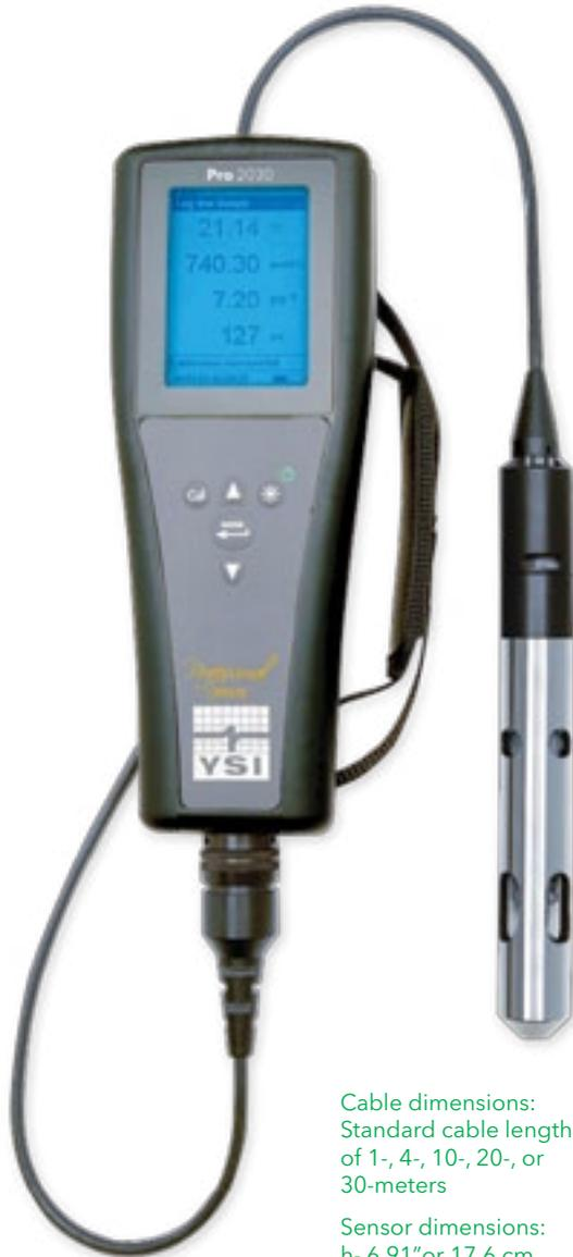
The YSI Pro2030 dissolved oxygen/conductivity instrument provides DO readings automatically compensated for changes in salinity. The internal barometer, Quick Cal feature, and simple interface make getting accurate data extremely simple.
