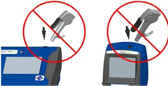
Figure 4-3: **DO NOT** Blow into Instrument
