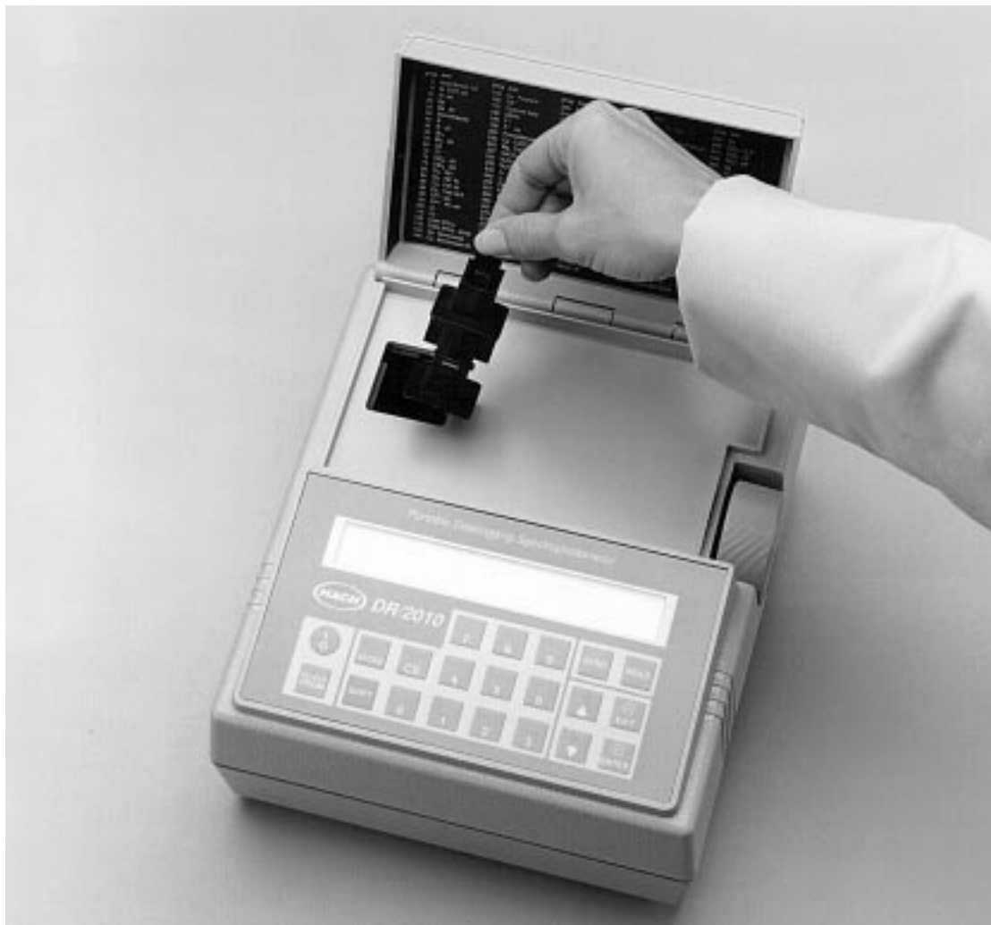
Figure 8 Installing the 1-cm Cell Adapter
