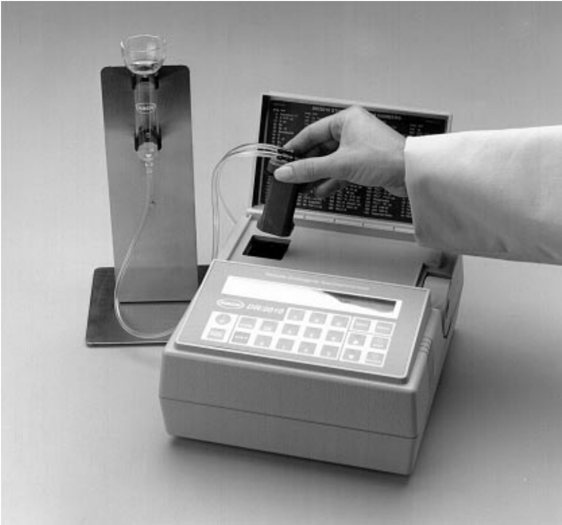
Figure 3 Installing the Pour-Thru Cell
