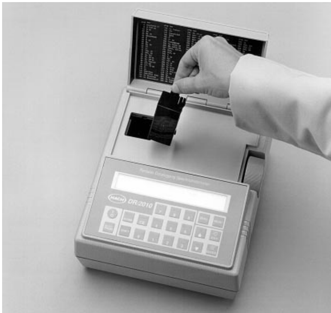
Figure 4 Installing AccuVac Vial Adapter
